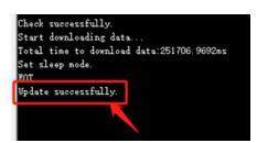
After finishing the update, cut off the PLC power, then power on the PLC again.
