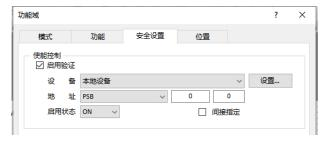
The bit limit can be set (the enabling state of the enable control can be customized). When the enabling condition is met, the component can be used normally (as shown in the figure above: when PSB0 is in the ON state and the trigger condition is met at the same time, the component can be used; if PSB0 is in the OFF state, the component is still unavailable even if the trigger condition is met).
