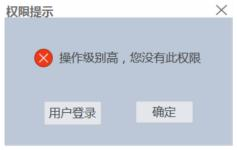
Click User Login, and it can be used normally after successful login. If the user has logged in and has this permission, he can directly operate the component without a prompt window.
