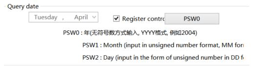
(2) Query by time period: Enter the start and end times to query, and after the query trigger bit is connected, the filtered results will be automatically displayed.
